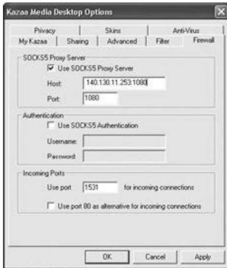
Figure 6-5: Using a proxy server with Kazaa to mask your IP address.
